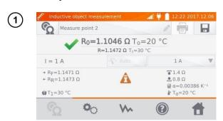
After finishing the measurement press .
