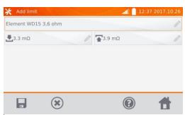
Use button to save the limit in the memory. Use button, to exit without saving.
