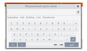
When necessary, name the measuring point.
