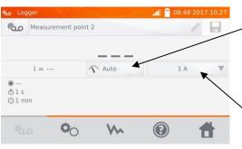
Switching between Auto/Manual mode: Auto - the measuring current is limited to a value not exceeding the set value, Manual - measuring current has the set value. When measuring inductive objects, only Auto mode is available.
