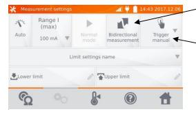
Switching Unidirectional/Bidirectional measurement.
