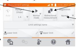
Switching Unidirectional/Bidirectional measurement.
